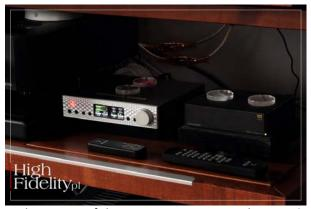
At the center of the system I set up was the Mytek player. I connected the tested product to its high quality USB input using a Curious Cables USB cable. Both devices were connected to the FunBox 3.0 router via LAN cables.
